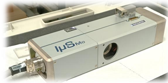
The Incoatec \mu\text{S} 1.0 (285x90x60 mm 3 , 3.5kg)
